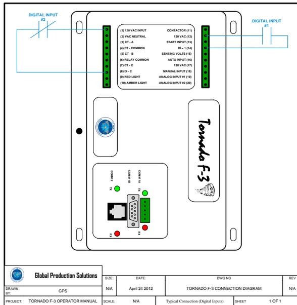
Figure 5 - Typical Digital Inputs
