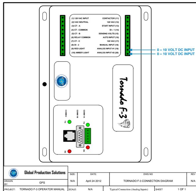
*Figure 6 - Typical Analog Input Connection*
